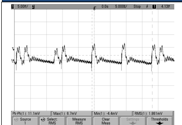
Ripple and Noise @25°C (Vin = 110V, Vout = nom., Iout = 0, Load = 0, ScopeBW = 20MHz)
